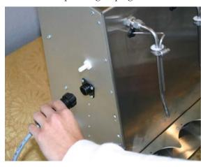
**3.** Plug the filler into a wall outlet. Turn on the Power Switch. DO NOT turn on the Pump Switch at this time.
