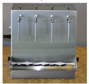
**2.** Unscrew the fixation screws holding the shelf to the bottom of the machine. Plug the electrical connector into the side of the filler (shown with optional gas sparge).
