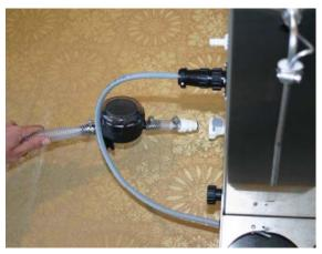
Note: To make sure there is no air in the flow path, turn the inline strainer upside down while the pump is running. This ensures that the air bubbles in the strainer housing mostly dissolves, although a little air bubble in the strainer is normal.
