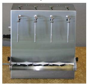
**2.** Unscrew the fixation knobs holding the shelf to the machine. Plug the shelf's electrical connector into the side of the filler (shown with optional gas sparge above the shelf connector).
