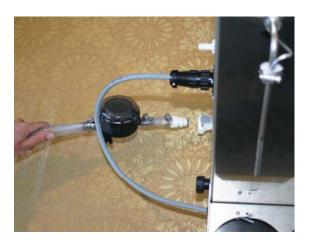
Note: To make sure there is minimal air in the flow path, turn the inline strainer upside down while the pump is running with 4 bottles in place. This ensures that the air bubbles in the strainer housing mostly dissolve, although a little air bubble in the strainer is normal.
