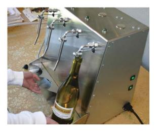
d. Note which holes on the side of the Machine are aligned between the filler body and the adjustable shelf. Install the fixation knobs to hold the shelf at this height.
