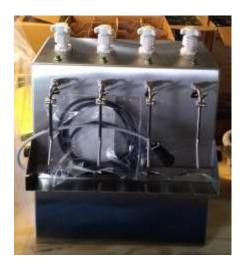
The four white valves on top of your unit are for flow control. Each valve controls the spout in which it is aligned. The valves functions are to increase or decrease flow per spout. Usually if foaming is occurring in your product, decreasing flow and or slowing down your flow will eliminate this problem.
