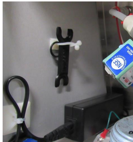
Push collet in with tool to remove hosing
