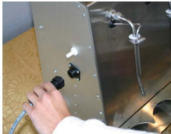
3. Plug the filler into a wall outlet. Turn on the Power Switch. DO NOT turn on the Pump Switch at this time.
