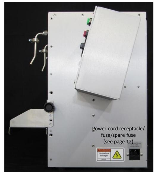
4. Place your bottles under each of the four spouts. Push the start button or hold the manual button to allow the pump to prime until you notice a consistent flow.
